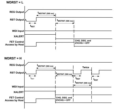
Figure 3. Watchdog Timing Chart – WDI Fault at Start-up
