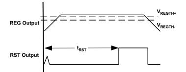
Figure 2. XRST Timing Chart – Power Up and Power Down
