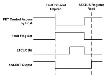
Figure 1. LTCLR and XLAERT Clear Timing
